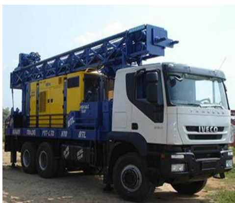
Water Well Rigs
